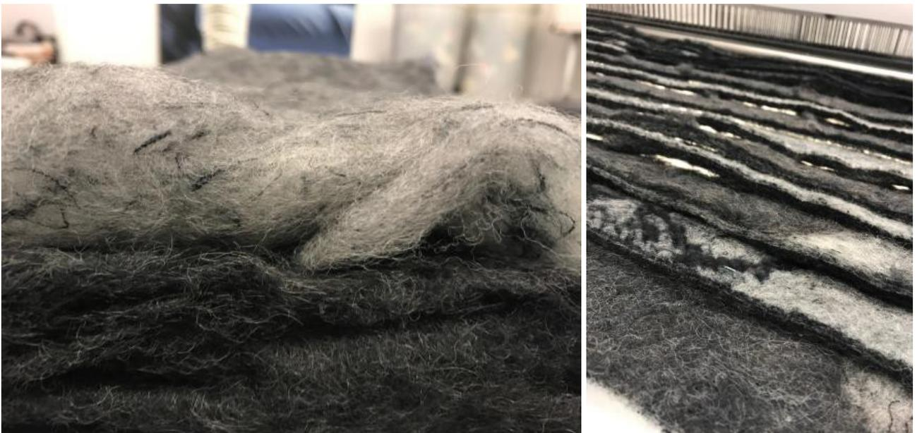
Fig 8 and 9. The fibres were blended with other recycled fibres from other waste streams, re-carded and felted.
